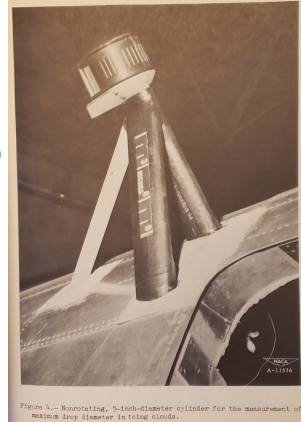
Figure 4. - Rotating, 5-inch-diameter cylinder for the measurement of maximum drop diameter in icing clouds.
